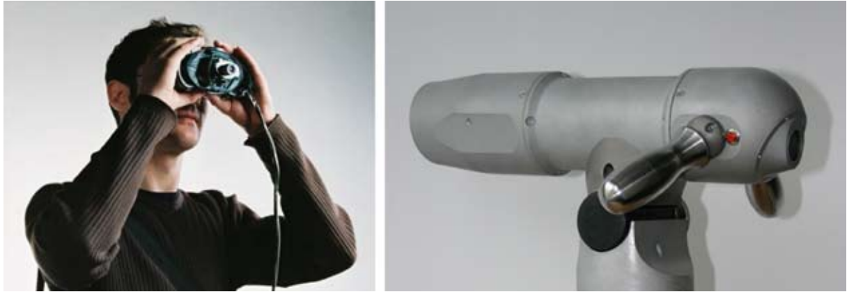
Fig. 11. AR devices: binoculars, (left) and telescope (right), through which the VR model is superimposed
